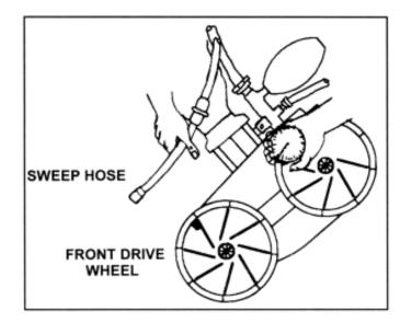
Have someone turn on pool pump and then booster pump while you place the Legend<sup>®</sup> Platinum in the pool just beneath the water surface. (Be sure to hold onto the Sweep Hose to avoid getting wet).
